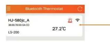
Click here to connect to the product. On this page, if you short press the defrost button on the controller, a red background will display a prompt. This function is used to identify the device when multiple devices are not connected
